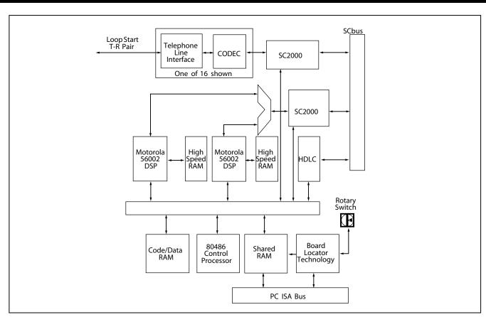
The D/160SC-LS board connects 16 analog (loop start) telephone lines to 16 on-board call processing resources or to other resources via the SCbus. This board provides:
