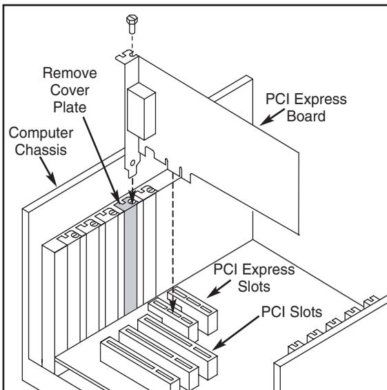
5. Reinstall the retaining screw.
