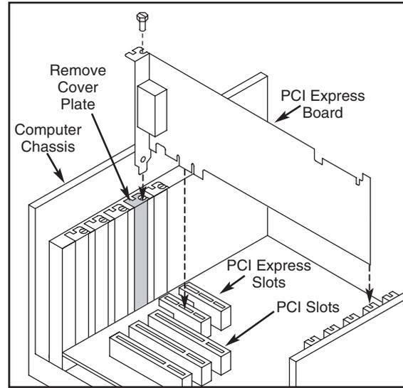
5. Reinstall the retaining screw.
