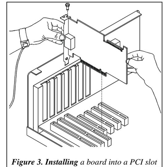
Figure 3. Installing a board into a PCI slot
