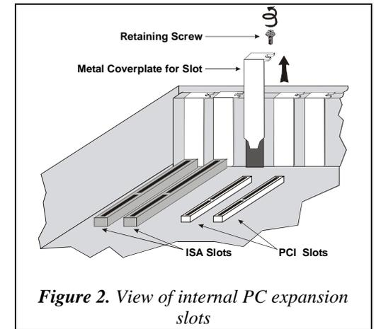
Figure 2. View of internal PC expansion slots
