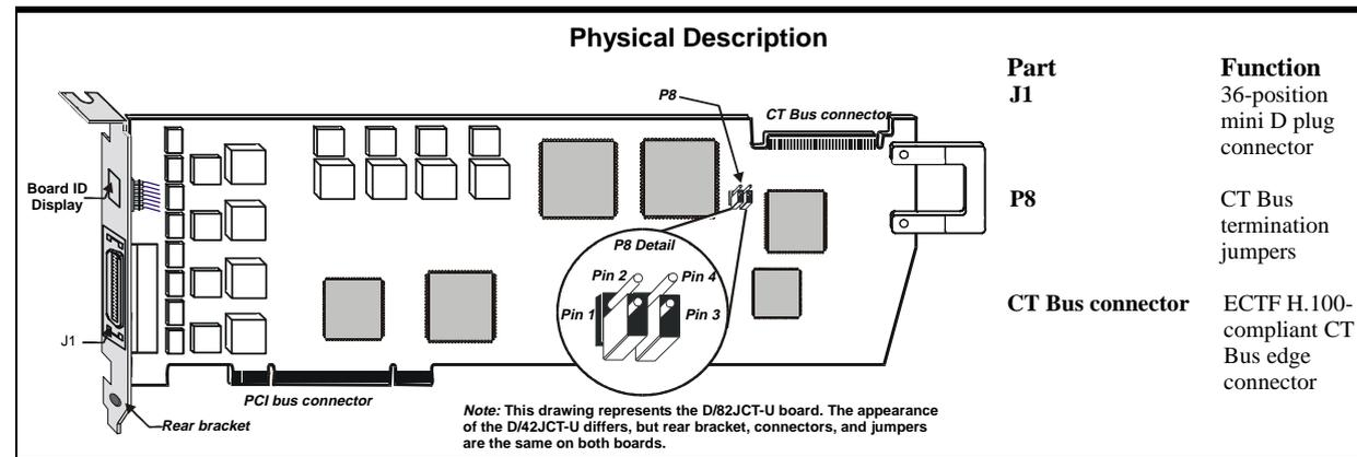
To give a PCI board with a rotary switch a Board ID other than 0, the rotary switch is set to the desired number. Because the PBX Integration boards have no rotary switch, the Dialogic Configuration Manager (DCM) software that is provided with the board automatically assigns Board IDs, beginning with 0, unless there are other PCI boards with a rotary switch settings of 0, 1, 2, etc. In that case, DCM would assign the first available Board ID not in use.
