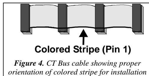
1. Attach the end connector on the ribbon cable to the CT Bus edge connector on the top edge of the first board. The connectors are designed to fit together one way only. If the connector does not seat fully on the board, turn the cable around and try again. Make sure that the colored stripe on the cable faces toward the rear bracket. (The stripe should be adjacent to pin 1 on the board connector.)
