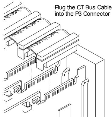
Plug the CT Bus cable into the P3 connector. To connect to the SCbus, use the CT Bus to SCbus adapter (Part Number 99-2446-001) and follow the instructions included with the adapter.
