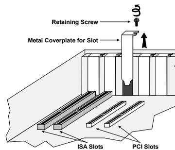
4. Insert the board's edge connector into the bus slot. Apply pressure only to the top edge of the board, and gently rock the board forward and backward to seat the edge connector into the slot.
