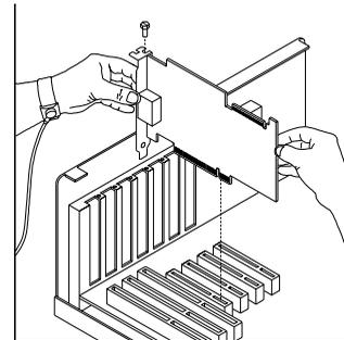
5. Install the retaining screw.
