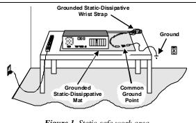
Figure 1. Static-safe work area
