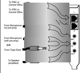
Figure 3. Bracket showing voice and audio connections
