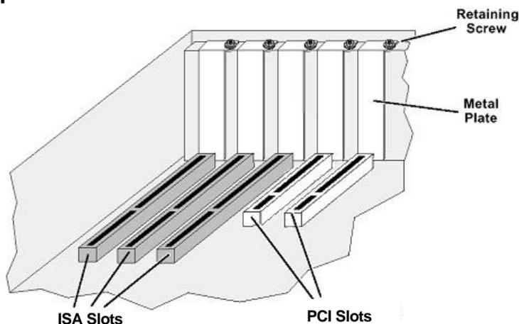
This illustration shows **ISA & PCI** slots. **ISA** slots are the longer of the two types and colored black. **PCI** slots are shorter and normally colored white, though they can be different colors such as purple on some motherboards. Insertion of the voice board will be the same for either type of slot.
