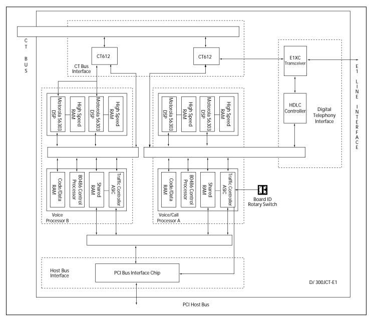
A DSP resource receives digital voice data via a CT612 module. The DSP processes the data based on SpringWare firmware loaded in its high-speed RAM. Each DSP performs the following signal analysis and operations on this incoming data:
