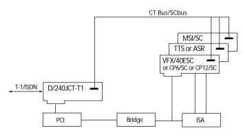
In a drop-and-insert configuration, use SingleSpan-JCT boards and a DTI™ board connected via the CT Bus/SCbus to pass T-1 or E-1 time slots through to each other. This configuration joins two separate T-1 or E-1 lines, or it can be placed in-line between a T-1 or E-1 line and a switch (a PBX, for example). Calls on individual channels can either terminate at a call processing resource on a SingleSpan-JCT series board, or "flow through" transparently to the DTI board.
