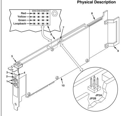
General Network Interface Alarm LED Power LED
