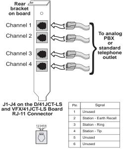
**Note:** Connect the Earth Recall signal to pin 2. Do not connect Tip or Ring lines to pin 2, or improper operation of the D/41JCT-LS-EW or VFX/41JCT-LS-EW will result.
